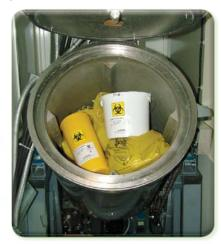
Select the required waste cycle on the 5,7 inch color touch-screen display and with pressing one button the door closes, the chamber rotates to the operating position and the waste cycle starts.
