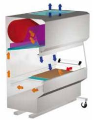
Airborne Particulate Cleanliness Class ISO 5, according to ISO 14644-1. 60% of the air volume is re-circulated, 40% is exhausted.
